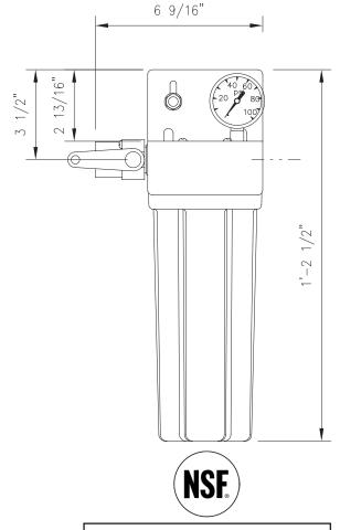
System is Tested and Certified by NSF International against NSF/ANSI Standard 42 Aesthetic Effects - Particulate Reduction (Class I) and the reduction of Chlorine, Taste and Odor.
