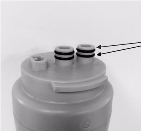
Lubricate all **four o-rings** with a good food grade silicon lubricant prior to installing the filter head.
