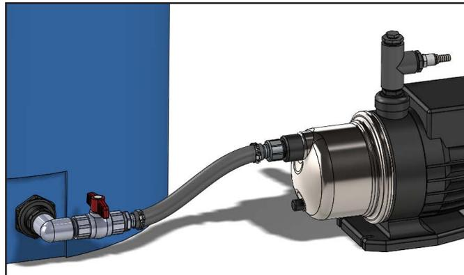
**Connecting 175 Gallon Storage Tank & RP Pump**
