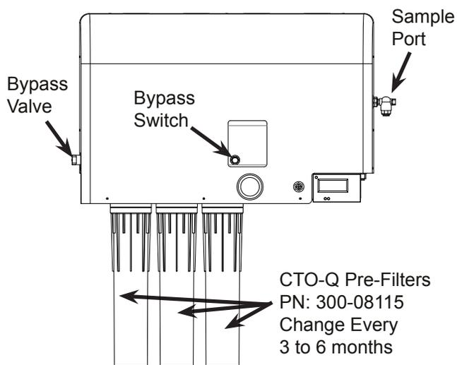
Normally, the most frequent routine maintenance required on the system is periodic replacement of the carbon/sediment pre-filters and the optional post-treatment cartridge. The CTO-Q cartridges should be changed every 1 month to 2 months, depending on water usage. In areas with high levels of sediment and other contaminants the CTO-Q cartridges may require more frequent changes.
