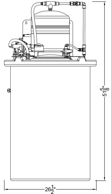
**IMPORTANT - ALLOW A MINIMUM OF 24" IN FRONT OF THE PROCESSOR FOR MAINTENANCE AND SERVICE. DO NOT MOUNT SYSTEM ABOVE THE CEILING OR IN A LOCATION THAT IS NOT EASILY ACCESSIBLE. WHEN THE 50 GAL. TANK ASSEMBLY IS FULL OF OPTIMIZED WATER IT WILL WEIGH 450 LBS (THE 175 GAL. TANK, 1500 LBS). ALWAYS LOCATE THE STORAGE TANK WHERE IT CAN BE ACCESSED DURING SERVICE.**
