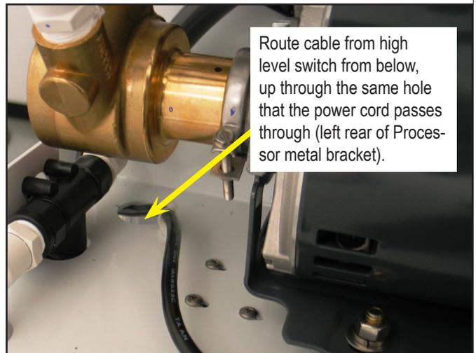
**Routing High Level Switch Cable**
