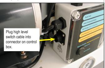
High Level Switch Cable Connection
