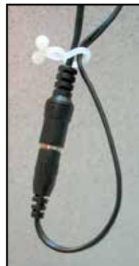
K. Twist clamp securing connected wires
